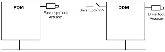
Figure 7. Structure of Central Door Lock System
