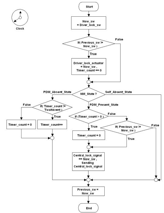
Figure8. Flowchart of Central Door Lock Function in Driver Door Module
