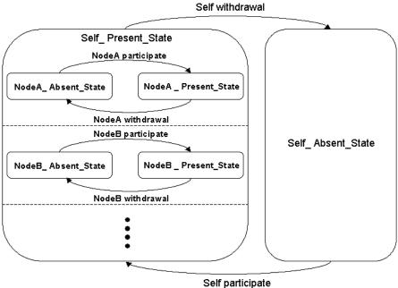
Figure 1. The State Diagram of OSEK-NM Design Attributes
