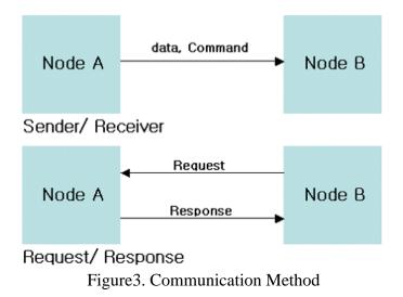
In the Request/Response method, two or more nodes exchange the information. Figure 4 illustrates the sequence chart and state chart for two nodes that establish Request/Response communication.
