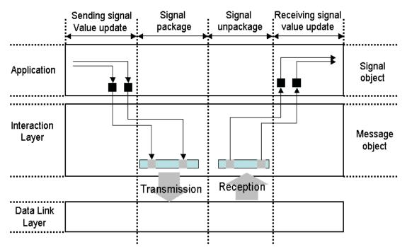
Figure2. Signal-Oriented Interface Using Interaction Layer
