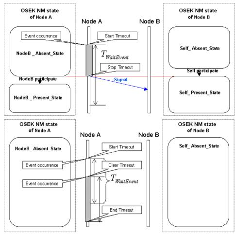
Figure6. Network Fault Countermeasure for Event Signal
